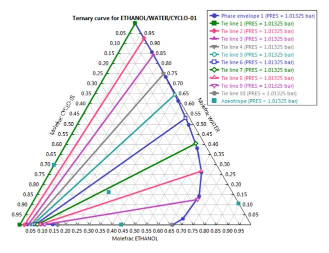
4.09. The squares on the diagram represent the compositions of azeotropes. There are 3 binary azeotropes and 1 ternary azeotrope. The phase envelope line represents the liquid-liquid equilibrium compositions.
