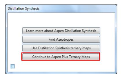
4.07. Click the **Continue to Aspen Plus Ternary Maps** button. The **Analysis | TERDI-1 | Input | Ternary Map** sheet is displayed. Select **Liquid-Liquid** for **Valid phases**. Enter **10** for **Number of tie lines** and **25** for **Temperature**.
