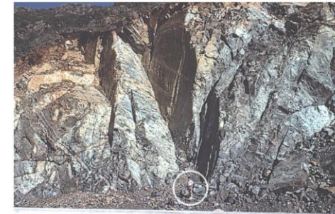
Figure 9.19 Planes of a wedge slide on a rocky slope in southern Spain.
