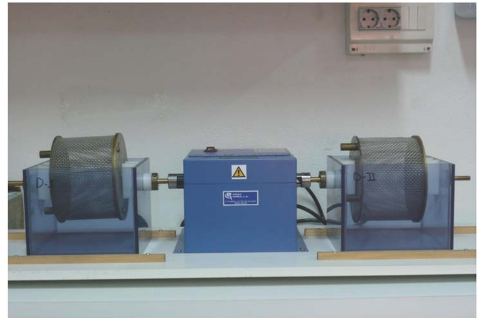
Figure 3.8 Slake durability test apparatus.
