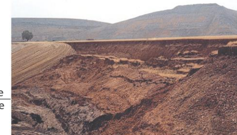
Figure 9.12 Curved failure in clays and shales in central Spain, showing the tension crack and vertical displacement of the slope head.
