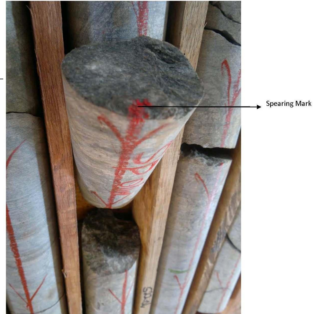
Fig. B.4 A run of broken core pieces is carefully re-assembled in a channel with the BOH mark against the straight channel edge. The channel should be at least as long as a standard core barrel (3–6 m). The one illustrated is one made from two lengths of 100 mm polypipe. The straight edge is used to draw the BOH line along the length of the core. An arrow pointing down-hole is drawn on one side of this line on to each core piece
