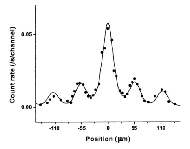
Diffraction pattern produced by scattering electrons from the standing light wave created by two opposed lasers.
